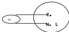
Voltmeter reading between N & E must be more than 100mV and less than 5V
